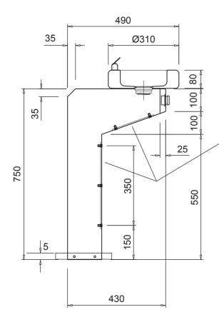
3mm S/S access panels fixed with M5 CSK security screws
