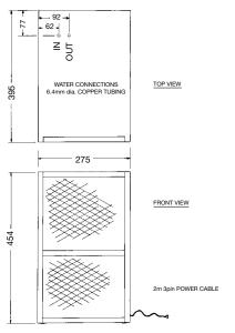
UNIT SUPPLIED WITH VENT & WATER CONNECTIONS
